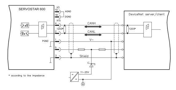
AGND and DGND (connector X3) must be joined together!
