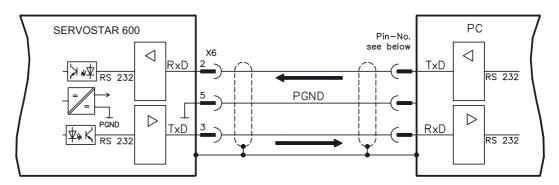
Interface cable between the PC and servo amplifiers of the SERVOSTAR 600 series:
