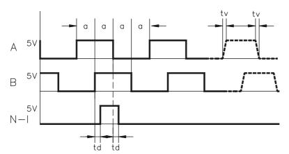
Edge spacing a  $\geq$  0,20  $\mu s$ Edge steepness tv  $\leq$  0.1  $\mu s$ Delay N-I-td  $\leq$  0.1  $\mu s$  $I\Delta UI \geq 2V/20 mA$
