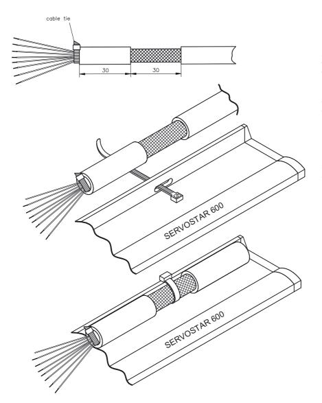
Remove the outer covering of the cable and the shielding braid from the cores for the required length. Secure the cores with a cable tie.
