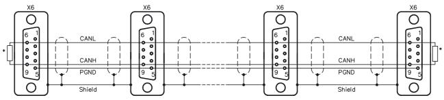
\* according to line impedance about  $120\,\Omega$
